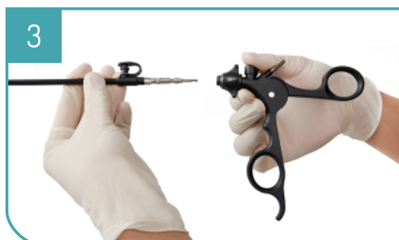
3 Engate o tubo na empunhadura aberta Engage the tube into the open handle
